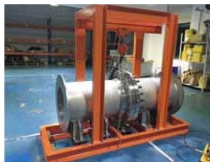
Figure2 試験治具(JPI Class300 24inch)
